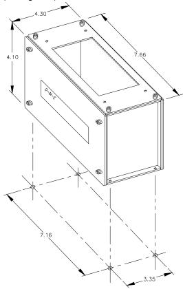
Figure 10 - Terminal Mounting Box Detail
