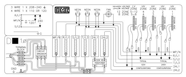
Figure 15 - Back Panel Wiring, Diagram D
