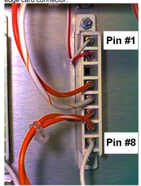
Figure 5 - Rear View of Edge Card
