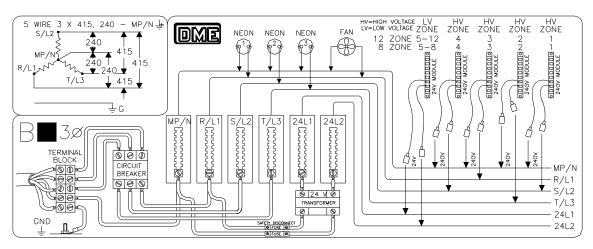
Figure 13 - Back Panel Wiring, Diagram B
