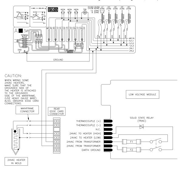
Figure 11 - Mold Wiring / Grounding
