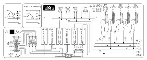
Figure 12 - Back Panel Wiring, Diagram A
