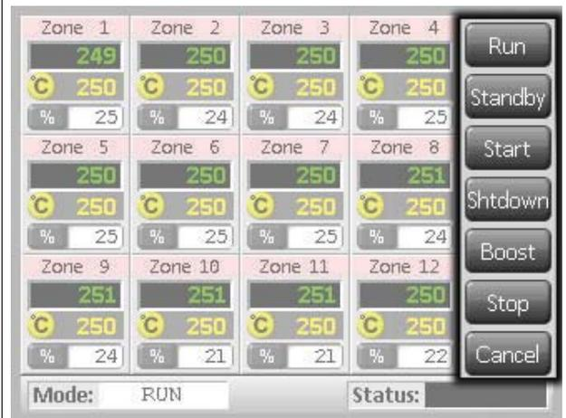
Secondary confirmation is required to go into any mode other than that which is currently being used.
