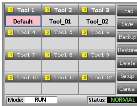
Touch **[Setup]** and enter system password to go to tool configure options
