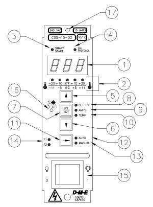
Figure 2 - CSS-15 Module (Note: CSS-30 Module is twice as wide as above; has circuit breaker instead of items 14 and 15)
