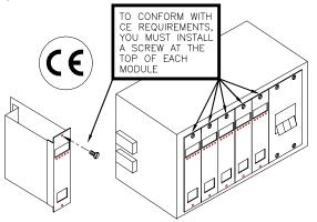
Figure 5 - CE Requirement (Add screw to the top of each module to conform to CE requirements)
