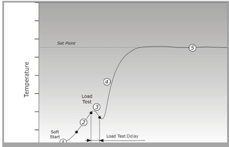
The zone controller slowly ramps up the heater power and simultaneously looks for a positive temperature change at the thermocouple input. The controller verifies the actual rate of rise against a predetermined value in program parameter r1. Power is slowly increased until the correct rate of rise is achieved.
