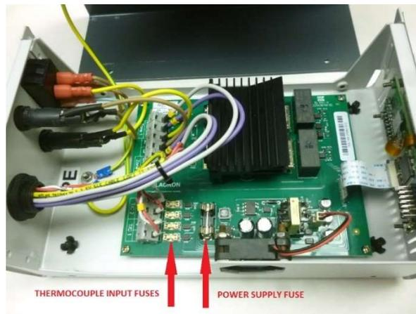
Figure 7-1 Fuse location inside the cabinet
