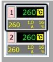
2. Use [**↑**] or [**↓**] to adjust the set temperature. You can hold the [**↑**] or [**↓**] buttons down to raise or lower value by large amounts.
