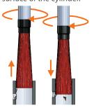
Stop brush rotation and remove brush while it is at rest
