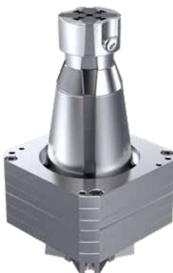
FIRST STAGE COLLAPSE (PARTIAL RELEASE OF UNDERCUT)
