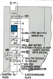
NOTE: When ejector plate is thicker than 1" connector may be centered on plate thickness. Altering mounting dimensions as required slot for lead wire should be depended as it approaches connector end as required.
