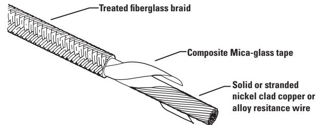
Best utilized: for wiring high temperature heating equipment, wiring and extensions for heating equipment used in plastic processing machinery. Well suited for presses and extruders, hot gates etc.
