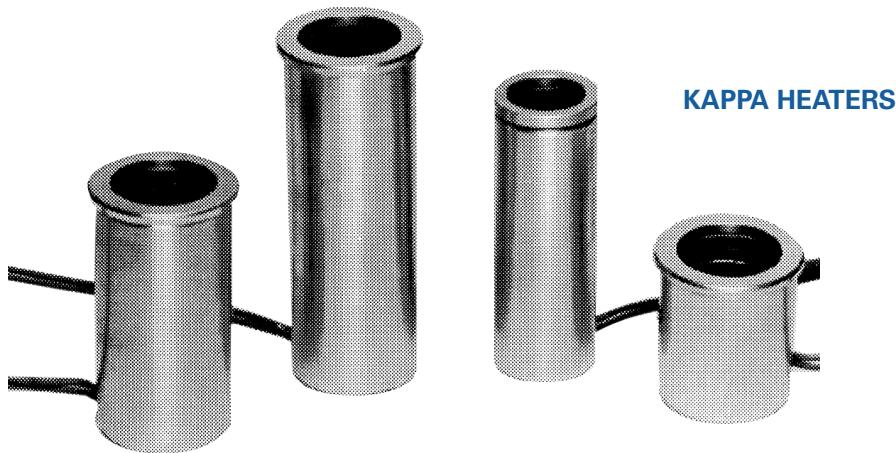
**The Kappa Series Heaters** are constructed with a nickel-plated copper inner sleeve and a stainless outer sleeve. The heater is tightly sandwiched between these sleeves eliminating the heat transfer problems associated with other dual-sleeved designs. The materials used direct the heat inward toward the nozzle, resulting in a very efficient heater with even heat distribution. The tightly-toleranced I.D. allows a slip fit with no clamping required.
