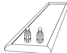
Post Terminals - parallel (side by side); minimum width  $\frac{3}{4}$ "
