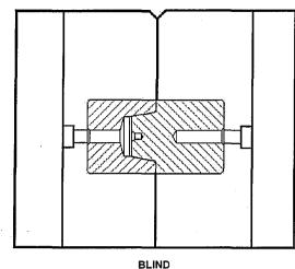
The above illustration shows three typical installations using DME tapered interlocks to suit different mold requirements. Shoulder plates are used with "through" construction, but not in "blind" pockets. Different "combinations" of through and blind construction may be used for a variety of applications.
