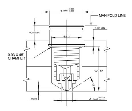
To compensate for the nozzle's growth when heat is applied, the linear expansion of the nozzle (BE) at a given temperature must be added to the nominal "A" dimension. The formula below shows how to figure boring depth (dimension "A" + BE). The tip of the nozzle will now be flush with cavity line.
