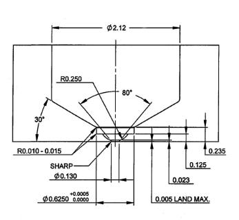
NOTE: Before installing a Point Gate Nozzle, it is important to take the nozzle's expansion factor into consideration. For best results, please follow the information below.
