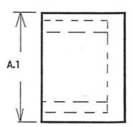
Plastic Cap with Internal Threads
