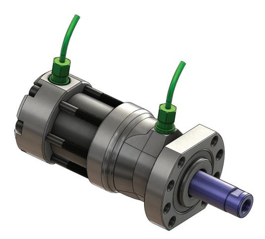
The DME Hydraulic Locking Core Pull Cylinder uses 3-wire, **induction** proximity sensors which require power in order to deliver a signal. Unlike classic mechanical-type switches, the inductive sensors have no moving parts. With the benefit of long life and excellent resilience and performance, these sensors are available in NPN (Standard) and PNP (upon request) types.
