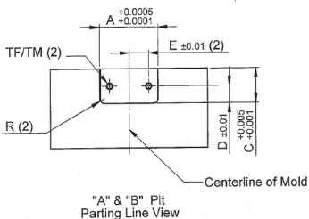
Recommended Pocket surface Finish: Ra 63 Dimensions shown in inches unless otherwise specified. Tolerances are:
