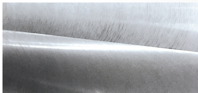
The milled stripes across the plate created by DME's state-of-the-art Fine-Milling technology. Surface Finish RA 90.
