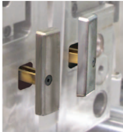
Quick Strip is actuated by the opening of the mold; reset by the closing of the mold.
