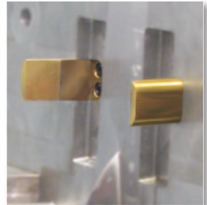
Quick Strip is actuated by the opening of the mold; reset by the closing of the mold.
