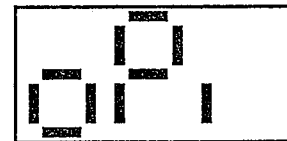
Figure 7. - Open Thermocouple, open input
