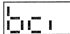
Figure 8. - Reversed Thermocouple, backward input
